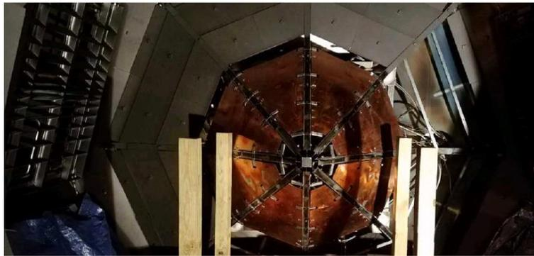
**Figure 12. Graphite conical beam dump and cooling system inside VTF-2**
