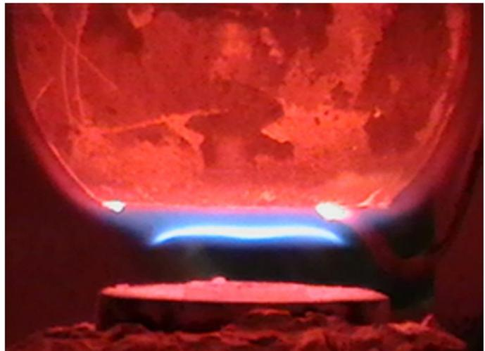
**Figure 6. CH<sub>4</sub>:C<sub>2</sub>H<sub>6</sub> (60:40) – air stagnation flame at 650 K, 5 atm ( $\Phi=1.0$ )**
