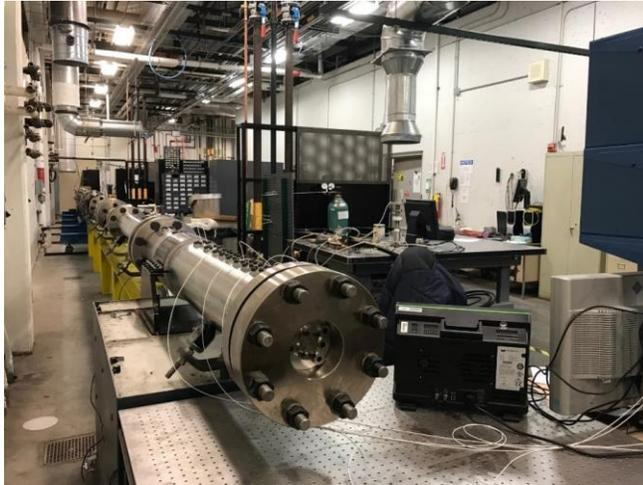
**Figure 7. The 69 ft shocktube at Georgia Tech**
