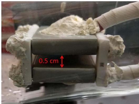
Fig. 5. Rectangular electrodes at 0.5-cm gap spacing.
